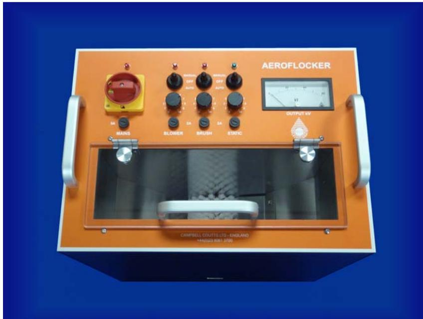
The flocking of objects which have deep recesses or sharp angles has always created problems for flock coaters. This is the result of the Faraday Cage effect where the electrostatically charged fibres are attracted to the nearest earthed surface which stops them reaching into cavities and corners.
